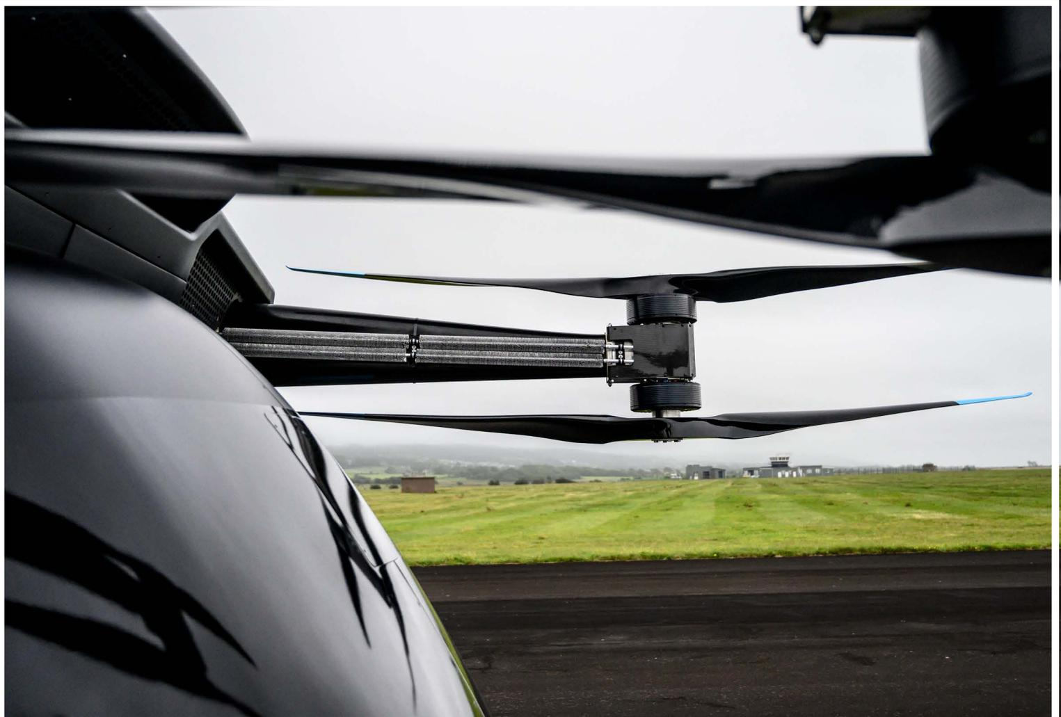
Vertical Aerospace is one of many companies working on designs for all-electric eVTOL aircraft with motors positioned by each of several open rotors.
