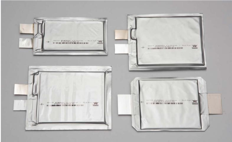
Oxis Energy is developing a lithium-sulfur (Li-S) battery it claims will allow electric aircraft to fly between 50 and 100 percent longer, with an output of 500 Watt-hour per kilogram.
