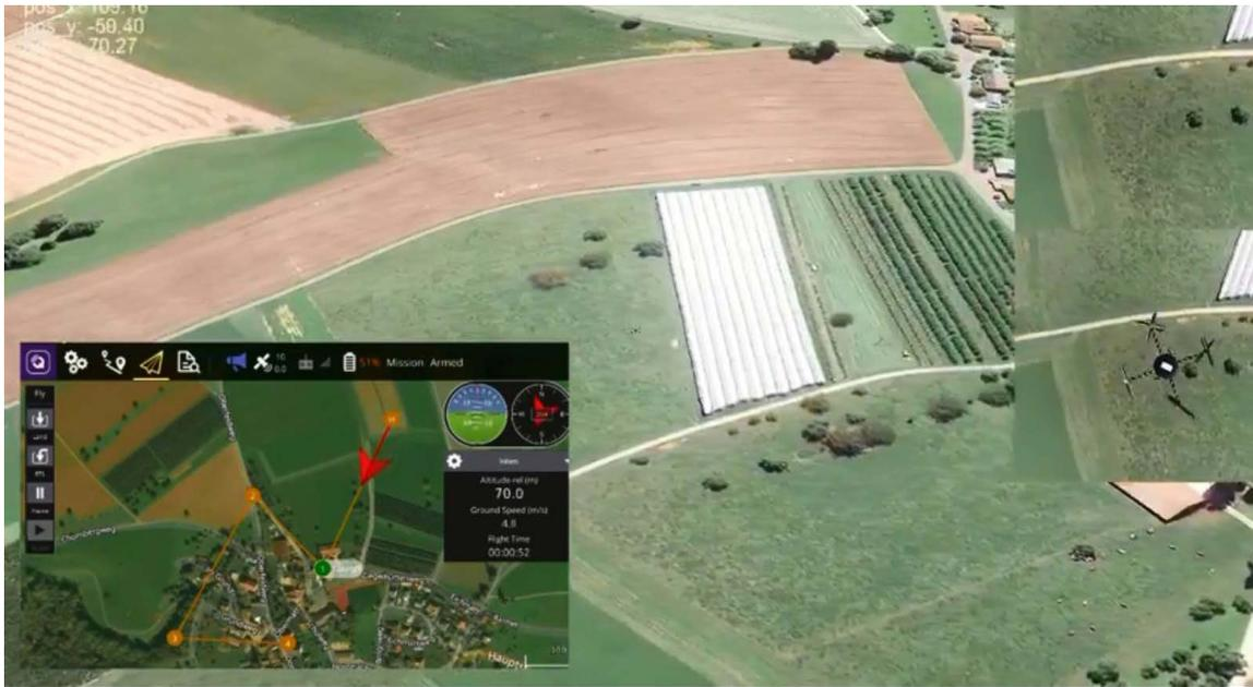
Swiss-based Daedalean is working on an artificial intelligence-based autopilot system using cameras to allow the flight control system to “see” everything that a pilot would see from the cockpit.
